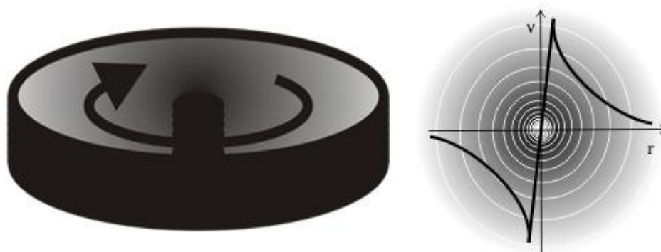
Figure 1.15. The change in the linear velocity of the vortex
